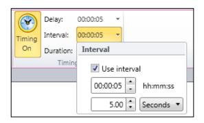
4. The measurement cycle (delay and interval) can be inputted and multiple cycles can be selected.
