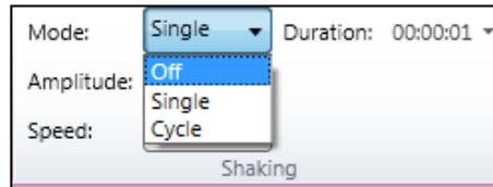
7. Select the amplitude (degree of linear shaking).
