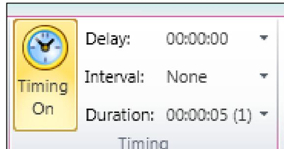
Users can then input the required kinetic parameters for a measurement cycle. The measurement cycle refers to the point of absorbance measurement including any timed delay and/or interval until the next reading.
