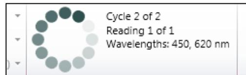
12. Results are displayed in each well. If dual wavelength measurements are carried out, absorbance measurements at both wavelengths are displayed. Absorbance measurements are also displayed on the bottom right hand panel if a well is selected.
