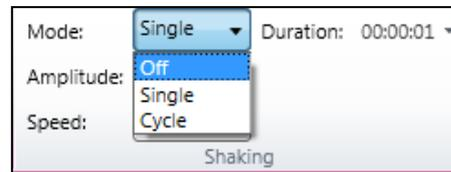
4. Select the amplitude (degree of linear shaking).
