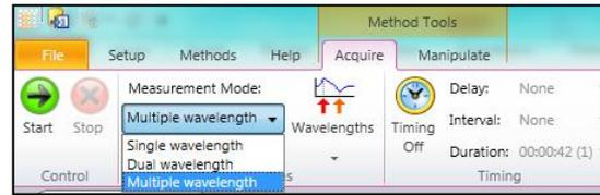
2. The menu is adjusted to allow users to select up to 4 wavelengths for measurement. Each wavelength must be different. For the EZ Read 800 Plus ELISA, users can input wavelengths of 405, 450, 492 and 620nm. For the EZ Read Research model, users can choose four wavelengths from 405, 450, 492, 562, 595 and 620nm. Click 'Start' to begin the measurement.
