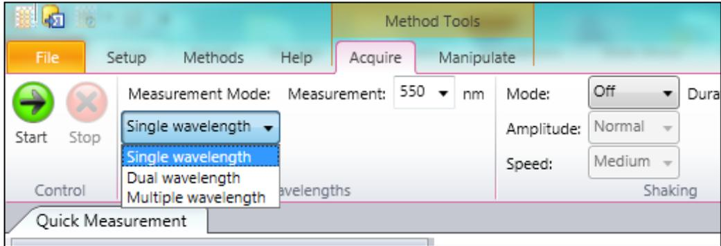
3. Users can also select to shake the microplate. Users can select shaking to be a single event or in timed cycles.
