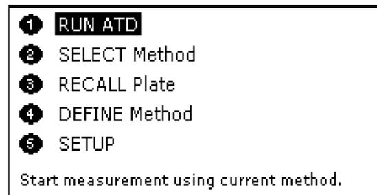
2. Press keypad directly below the corresponding option on the display (F1, F2, F3 and F4) to select the appropriate option.
