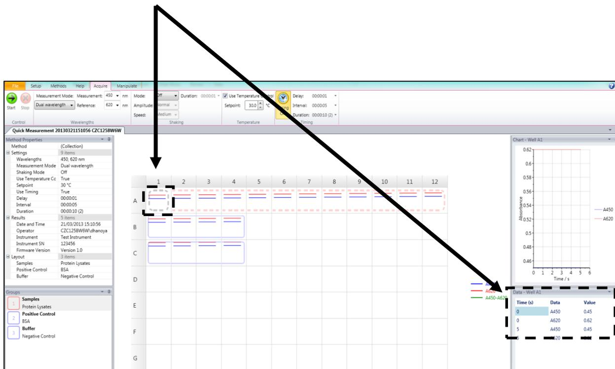
The lines shown in each well refer to the measurement at one wavelength over time. Different wavelengths used for absorbance measurements are assigned a specific colour and identified by a legend.
