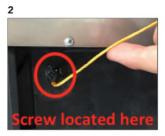
Carefully follow the orange string that is attached to the red transport clip to underneath the unit to remove a screw. Carefully move or tilt the instrument away from the table to see the screw located underneath the unit.
