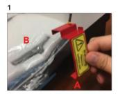
After removing the instrument from the packaging, please set the instrument on a level surface. Remove the red transport clip from the front of the instrument. (A) Remove the styrofoam plastic bag. (B)
